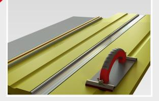
Press the external part of the Thermo-WINDOWSILL in the prepared, assembled window set.
