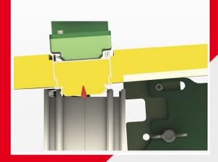
During pressing in, pay a great attention to the setting of the Thermo-PANEL's lower clasp and the internal part of the window frame's profile. They should be in alignment with each other.
