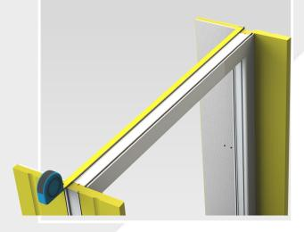
After applying the adhesive sealant and adhesive , press the upper Thermo -PANEL in the window frame 's profile , making sure the edges of the upper Thermo -PANEL are in alignment with the side Thermo-PANELs.
