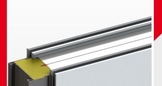
Cut the side Thermo -PANELs to the length measured from internal part of the window frame to internal part of the Thermo -PROFILE , remembering that the length of Thermo -PANEL should be measured from the internal part of the sealing clasp.
